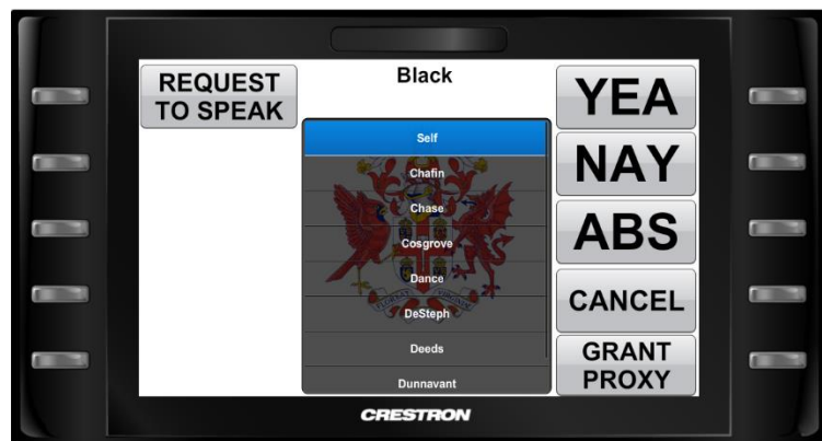
Example of Committee Voting System Touch screen Showing Senators who have granted Sen. Black their proxy to vote; this list may be scrolled by "swiping", similar to a smartphone. Similar functionality may be used to display Request to Speak queues or other information.
